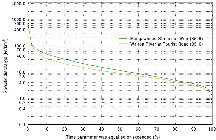
Figure 11.6: Flow duration curves for two Hunua area surface water catchments.
