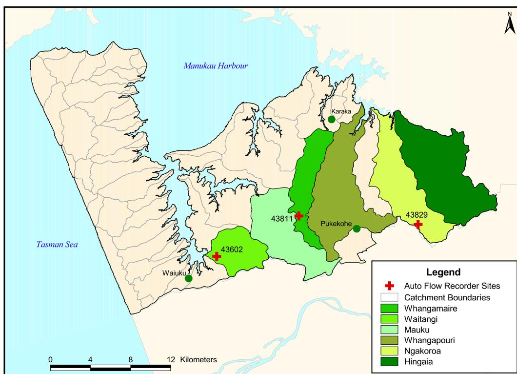
Figure 12.4: Surface water catchments and flow monitoring sites in the South Auckland area. The six key surface water catchments are indicated.
