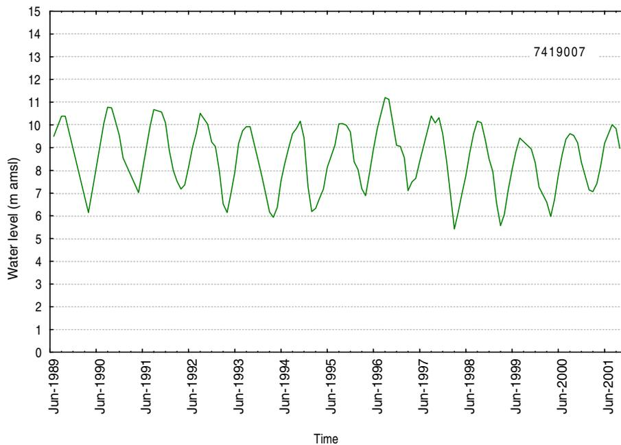
Figure 12.9: Groundwater level record at Fielding Road sand (7419007) monitoring bore.
