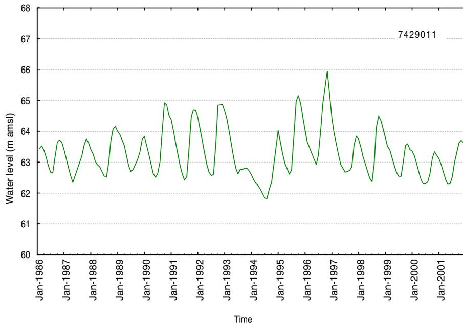
Figure 12.8: Groundwater level record at Revell Court (7429011) monitoring bore.
