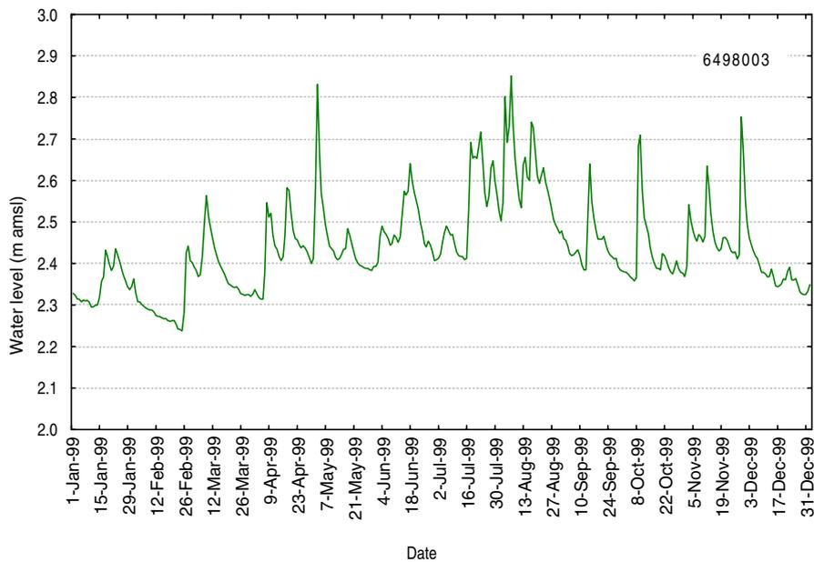
Figure 10.9: 1999 groundwater levels at Angle Street (6498003) showing the rapid response to recharge events.
