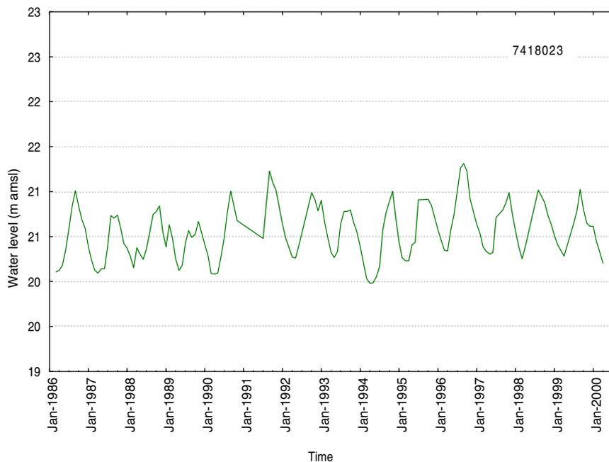
Figure 12.10: Kaawa Aquifer groundwater level record at Batty Road (7418023) monitoring bore.
