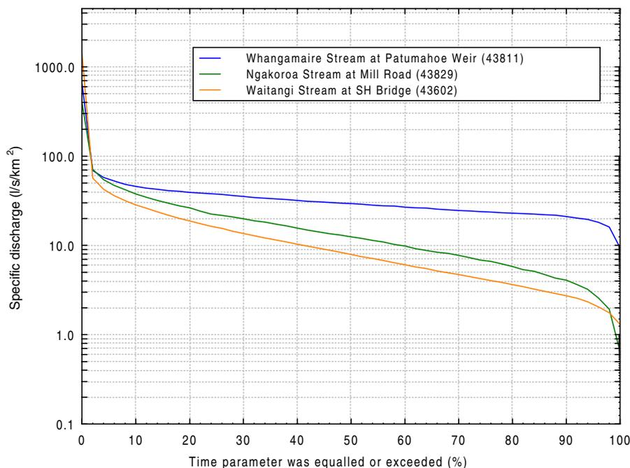
Figure 12.5: Flow duration curves for three South Auckland area surface water catchments.
