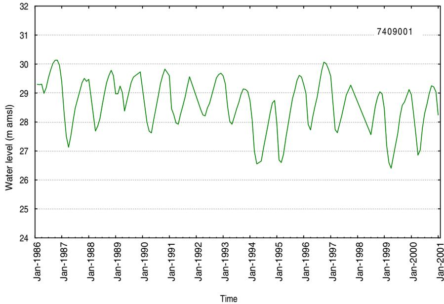
Figure 10.11: Groundwater level record at Burnside Road (7409001) monitoring bore.
